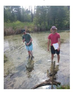
The site chosen for the test run data collection was about 100' downstream from the County Road 100 bridge where the stream bottom was relatively flat and the Cut was approximately 36' wide. A sturdy stake was driven into the west bank at the water's edge to serve as the zero point for subsequent measurements. Seven bamboo garden stakes were placed in the stream at 5' intervals to define the cells for area between the stakes and define where to measure average water velocity through each cell.
