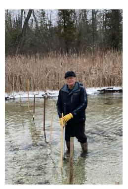
**Flow rate January 8, 2024** was determined to be 34 cubic feet/second. Measurements were taken by Becky Gibson and Fred Swinehart.
