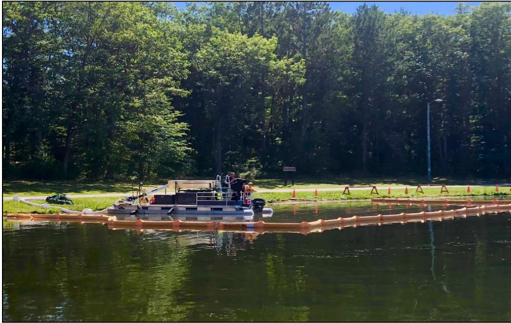
Figure 59. A DASH boat used in the South State Park Lagoon for aquatic plant removal.
