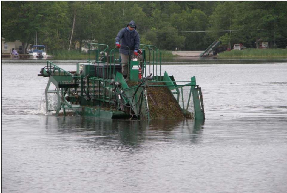
Figure 53. A mechanical harvester used to remove aquatic plants.
