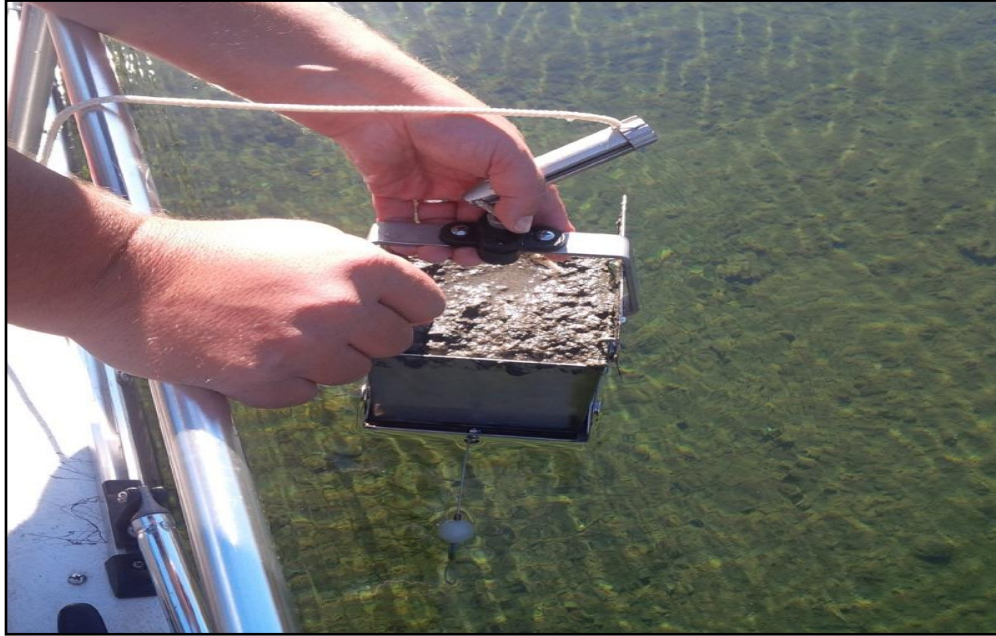
Figure 42. An Ekman hand dredge for sampling lake sediments.
