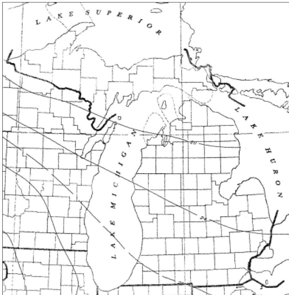
Figure 2 – May - October evaporation (in inches) from an open water surface
